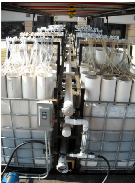
Figure 20: Mobile fracture water preparation / flow back water concentration unit. Taken from [47]
