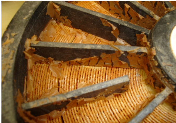
Figure 2: Iron fouling feed of a lead element
